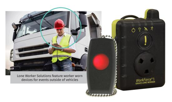
These Lone Worker Solutions interface with the vehicle's tracking unit, providing live information, including the location of the driver and vehicle at the time of the triggered event. Alerts can be sent to nominated recipients to follow a defined procedure or be diverted directly to emergency responders. This system allows operators to enhance the safety of their drivers whilst ensuring Chain of Responsibility compliance.
